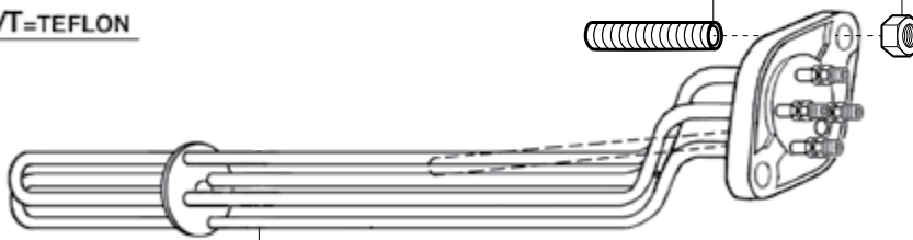
575123= GR1-2 3000W 220V 260mm 630090/22= GR2 3500W 220V 390mm 633004/22= GR3 3700W 220V 580mm
